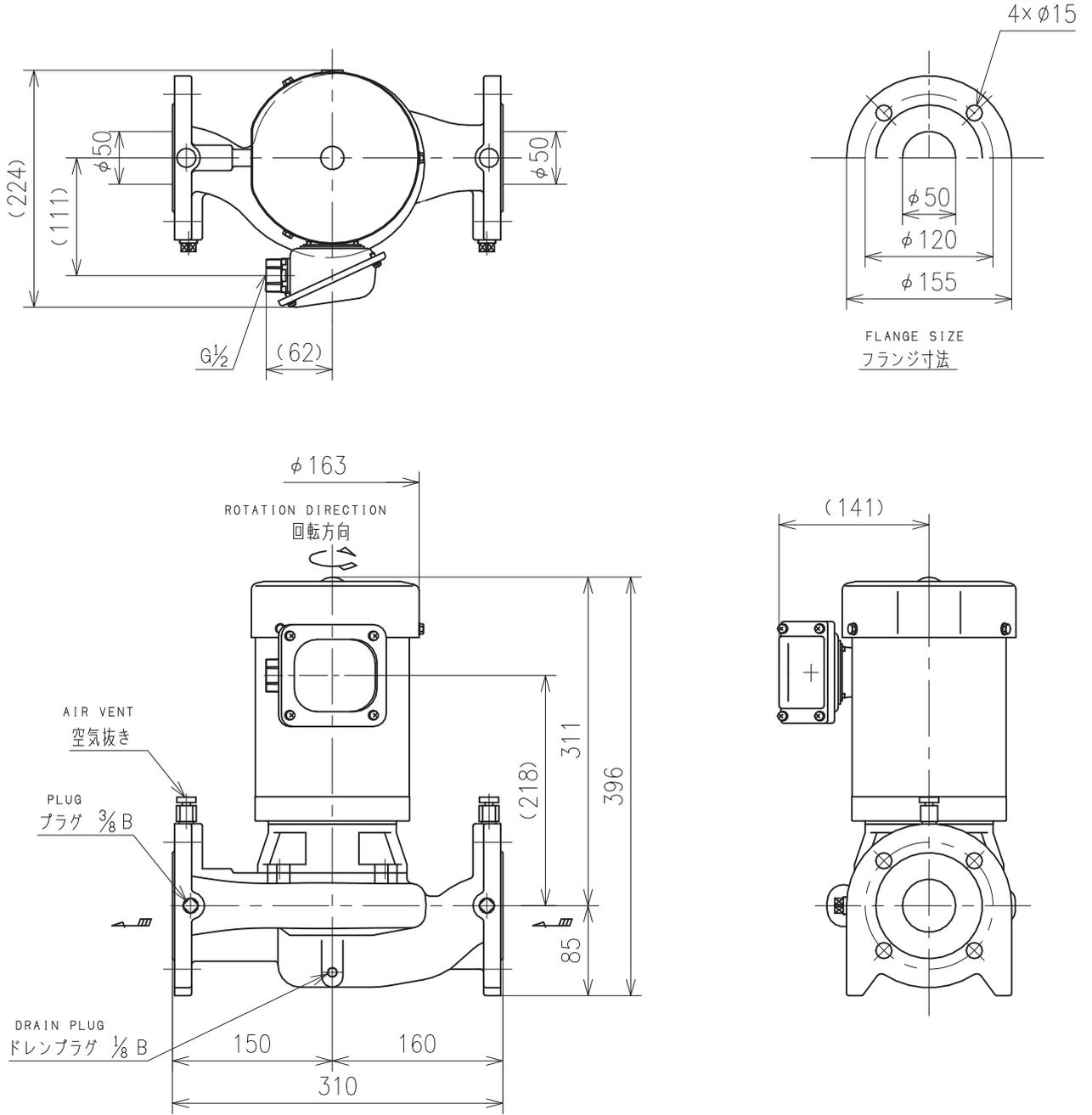
Flange size is conformed to JIS 10K thin type.
