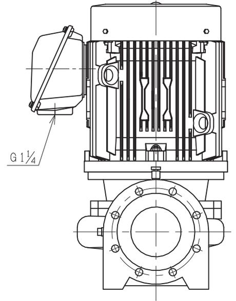
Flange size is conformed to JIS 10K thin type.
